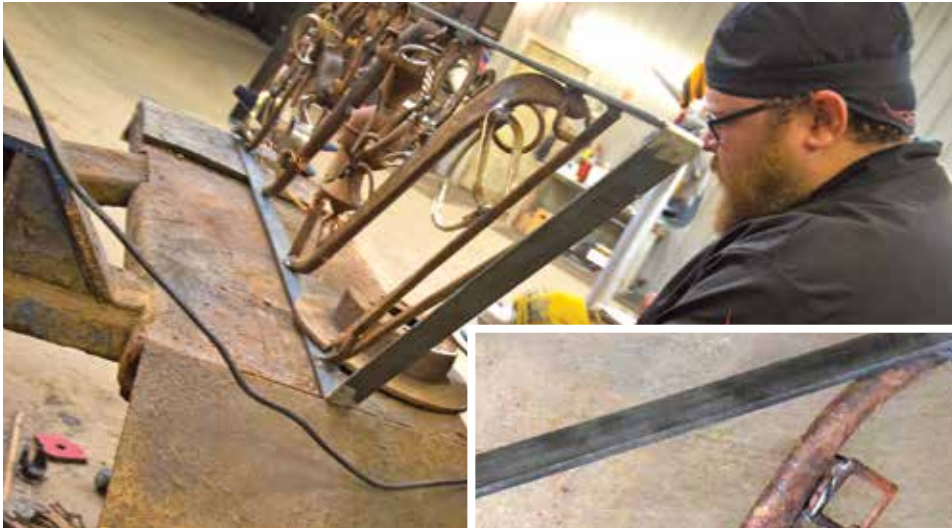
In these 3 photos, Josh works to complete a custom banister and rail filler for a new home. Made of various memorable farm parts supplied by the customer, the filler brings to life “touch and feel” memories of their past. The rail consists of stirrups, horse shoes, belts, buckles, small bells, and various other parts traditionally found in old barns and stables.
